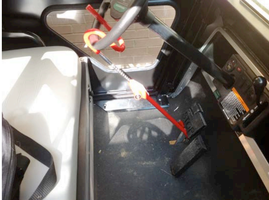
Properly engaged anti-theft brake-steering wheel lock for the golf carts. Photograph courtesy of Dr. Zane Mitchell (2015).
